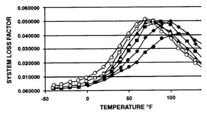
**Test Method:** The following data were obtained by doing a frequency sweep from 1 to 100 radians/sec (0.16 to 16 Hz) at 5 different temperatures:  $-20^{\circ}$ ,  $10^{\circ}$ ,  $0^{\circ}$ ,  $10^{\circ}$ , and  $22^{\circ}$ C. A 3 point bend geometry was used on the Rheometics RSA II. Time – temperature superposition was used to create the master curve for a reference temperature of  $22^{\circ}$ C.
